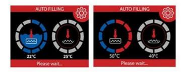
When the boiler gets to 60C, heated water is sent to the washing tank. This process continues until the washing tank is fully filled.
