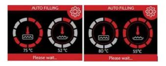
Note: The washing process will not start until the Washing tank and Boiler reach the set temperature
