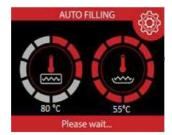
After the washing tank is fully filled, the machine waits for the boiler and washing tank set temperatures to be reached. When the Boiler water temperature reaches 85C and the Tank water temperature reaches 55C the machine is ready for washing.
