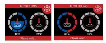
When the boiler gets to 60C, heated water is sent to the washing tank. This process continues until the washing tank is fully filled.
