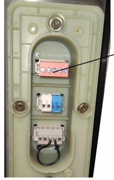
Note: Maximum current drain at the transfer strip: 0.5 A. Only connect external dosing devices with their own fuse protection. Include the dosing device in the protective circuit (PE) of the warewasher.
