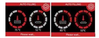
Note: The washing process will not start until the Washing tank and Boiler reach the set temperature
