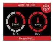
After the washing tank is fully filled, the machine waits for the boiler and washing tank set temperatures to be reached. When the Boiler water temperature reaches 85C and the Tank water temperature reaches 55C the machine is ready for washing.
